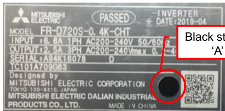
Product serial number plate (up to 3.7kW) Repair identified by Black sticker 'A'
