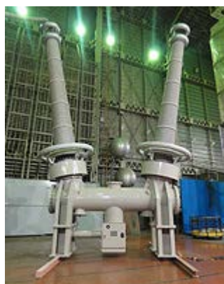
Gas circuit breaker
