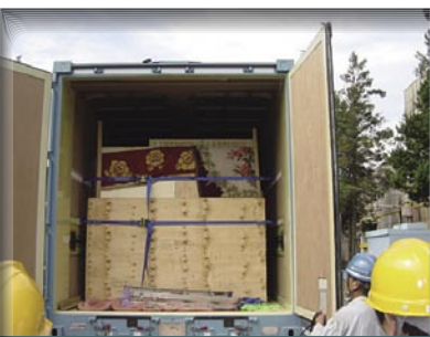
Belts are used to tie down products packaged in cardboard boxes, which tend to shift during transport.
