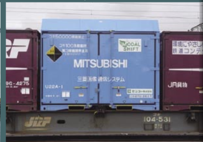
Containers with high ceilings are used to transport products stacked up to 2.4 meters.
