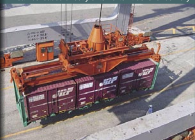
Three 12-foot containers, transported on flat-bed trucks, are easily packed into 40-foot shipping containers for oversea transport. The 12-foot containers can then be conveniently transported by rail at the other end of their ocean voyage.
