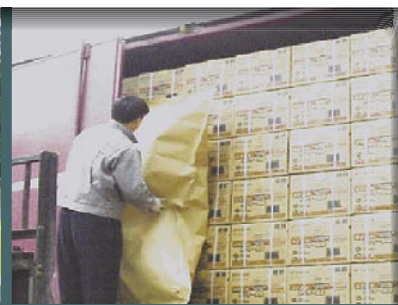
Airbags are used to package products tightly and eliminate excess air space.
