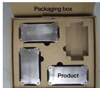
To cushion products against shock during shipment, we have designed a new type of packaging for semiconductor power modules, for which over-spec packaging is common. The new packaging cushions the modules at the corners—thereby maintaining the box shape—while using rolled cardboard materials. This compactness reduces cardboard material requirements by 51%.
