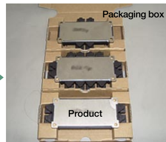
To cushion products against shock during shipment, we have designed a new type of packaging for semiconductor power modules, for which over-spec packaging is common. The new packaging cushions the modules at the corners—thereby maintaining the box shape—while using rolled cardboard materials. This compactness reduces cardboard material requirements by 51%.
