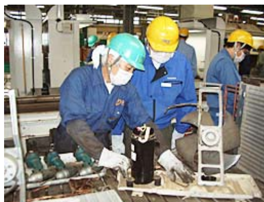
Appliance disassembly at Hyper Cycle Systems (In learning design for the environment, product design personnel receive guidance from appliance disassembly line veterans.)
