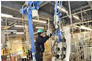
Refrigerator disassembly line Upright position is an innovative technique ensuring speed and efficiency
