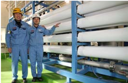
Water detoxified by microfiltration. It is further filtered by reverse osmosis (RO), which eliminates impurities like soluble salt. The water is used again for washing at the metal plating factory.
