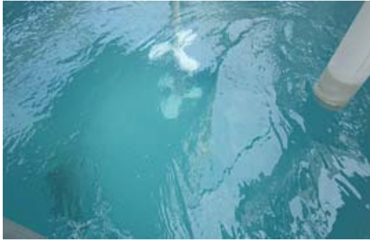
Water detoxified by microfiltration. It is further filtered by reverse osmosis (RO), which eliminates impurities like soluble salt. The water is used again for washing at the metal plating factory.
