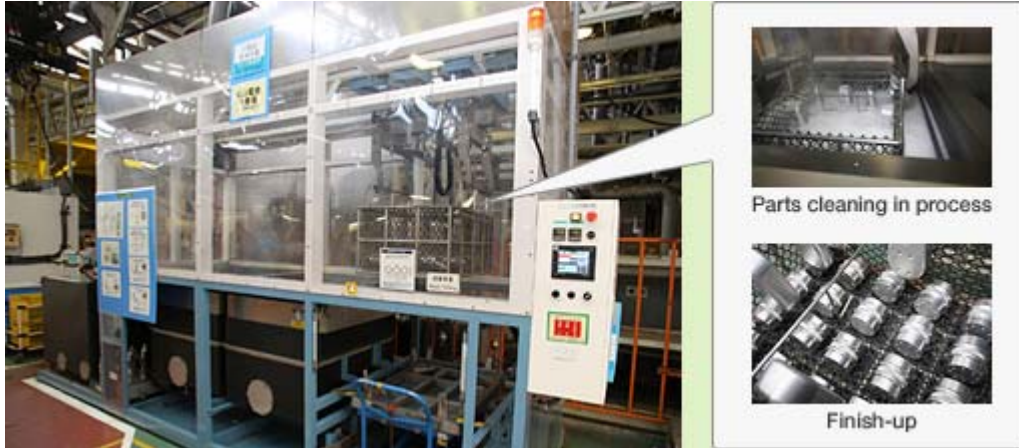
Microbubble cleaning equipment
