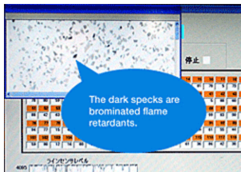
Award-winning technology where X-rays detect chips containing flame retardant in the granulated plastics mixture, and 124 individual air guns are instantly instructed to blow them aside.
